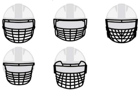
As a general principle, any facemask with five or more horizontal bars below the eyes is not permissible. The exception is the facemask below - because of the larger gap between bars 2 and 3 and between 4 and 5, it is permissible.
